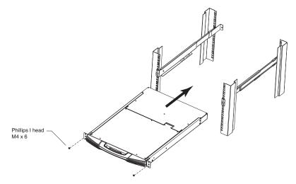
4. Slide the rear attachment sliding brackets along the slide bars until they contact the rear of the KL1116, then use the screws supplied with this package to attach the bars to the rear of the KL1116 (tighten the screws all the way).
